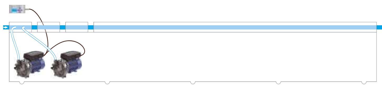
Installation example for controlling a pressure level with two vacuum units via the software function master slave
